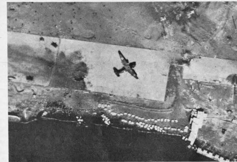
New flying boat, Ibusuki Field 82 has a parasol wing, single tail assembly. Wing is straight along leading edge, and inboard trailing edge, making it look swept-forward.
